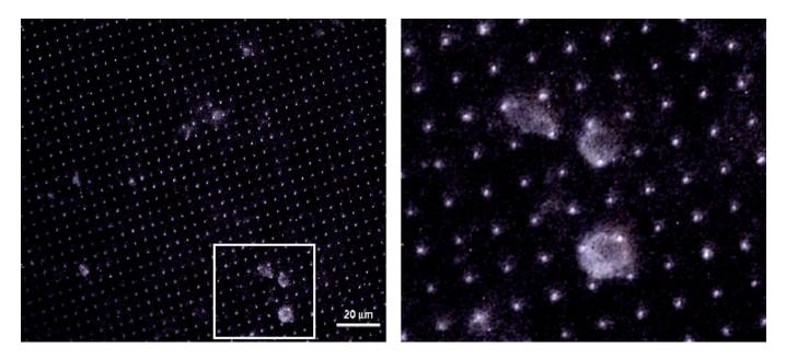
An array of silicon microneedles (200nm diameter), on a silicon wafer showing the adhesion of biological material. This image was taken in ambient conditions, with no sample preparation. The zoomed-in region on the right reveals membrane contours and points of adhesion between the cells and the microneedle structures. Distortion of the cellular membrane is evidence of the strong binding of the substrate to the needles. (Scale bar =  $20 \mu m$ )
