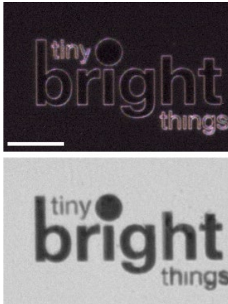
HalolImage and brightfield image for a nanofabricated pattern formed by depositing a 50 nm thick gold film. (Scale bar = 20 \mu m)
